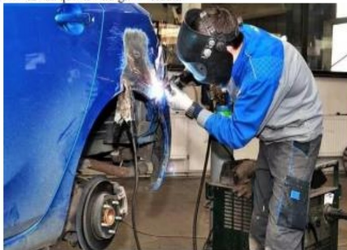
2-rasm. Avtomobil kuzovlarini payvandlash
