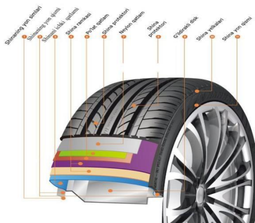
2.2.1-rasm. Avtomobil shinalarini tuzulishi [2]
