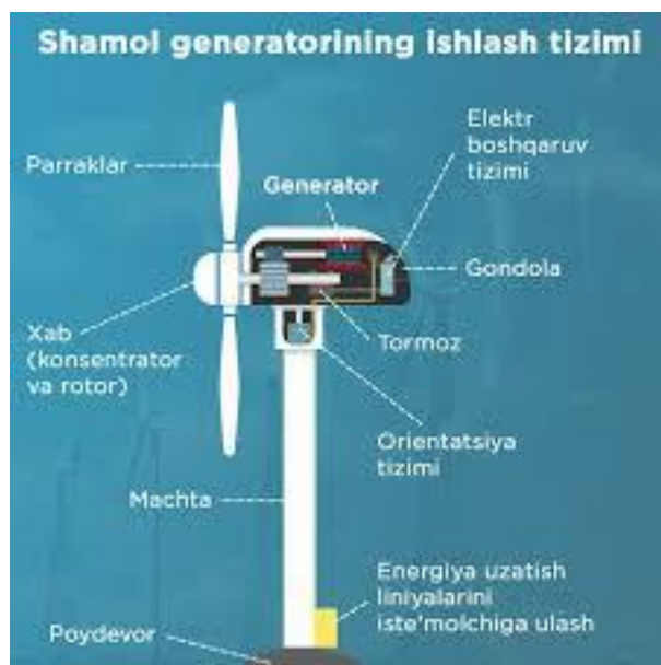
1-rasm . Shamol generatorining ishlash tizimi .
