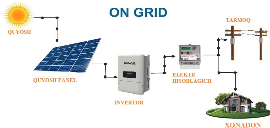
1-rasm. ON-GRID tizimli FESning ulanish sxemasi
