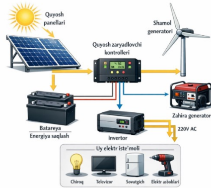
Figure 2. Autonomous photovoltaic power plant scheme
