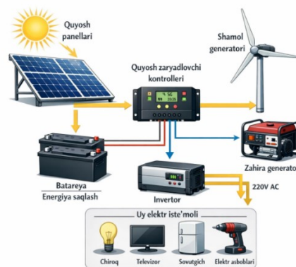
Figure 2. Autonomous photovoltaic power plant scheme
