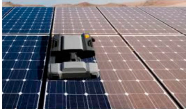
1-rasm. Quyosh panel yuzasining changdan tozalanish jarayoni
